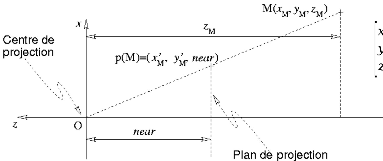
$$\begin{bmatrix} x_{M'} \\ y_{M'} \\ z_{M'} \end{bmatrix} = \begin{bmatrix} \frac{x_M}{(z_m/near)} \\ y_M \\ \frac{(z_m/near)}{near} \end{bmatrix}$$
